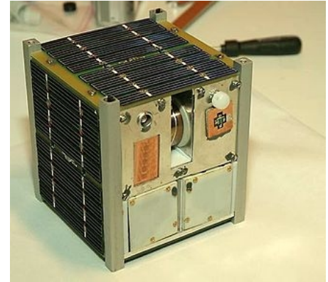
Steps towards satellite's miniaturization: Ncube-2, a Norwegian CubeSat (10 cm (3.9 in) cube). Source: Bjørn Pedersen.
